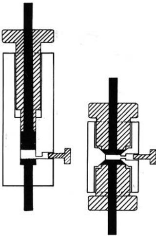
**FIGURE 3.** Macrochamber: left, for changing the volume continuously; right, for a fixed volume (black, stainless steel electrodes).
